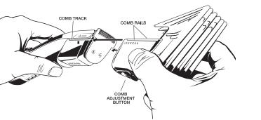
To attach comb to clipper, align <u>both</u> comb rails with the comb tracks on both sides of the clipper and slide into place. Once comb is secure you will hear a click sound, letting you know it is locked in. Ensure comb is properly secured by pushing down on comb, the comb should not slip. To adjust comb height press down on the comb adjustment button and slide up or down as necessary.
