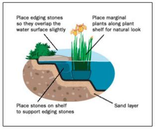
Well-constructed, natural-looking ponds have stable stone edging and no liner showing above the water level. Pond water levels do drop during warm, dry weather, however. For that reason, stones should be used to hide the liner, several inches below the water surface, so that the liner will remain unseen.
